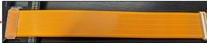
Flex cable carries 64 anodes, shared cathode, and temperature probe lines
